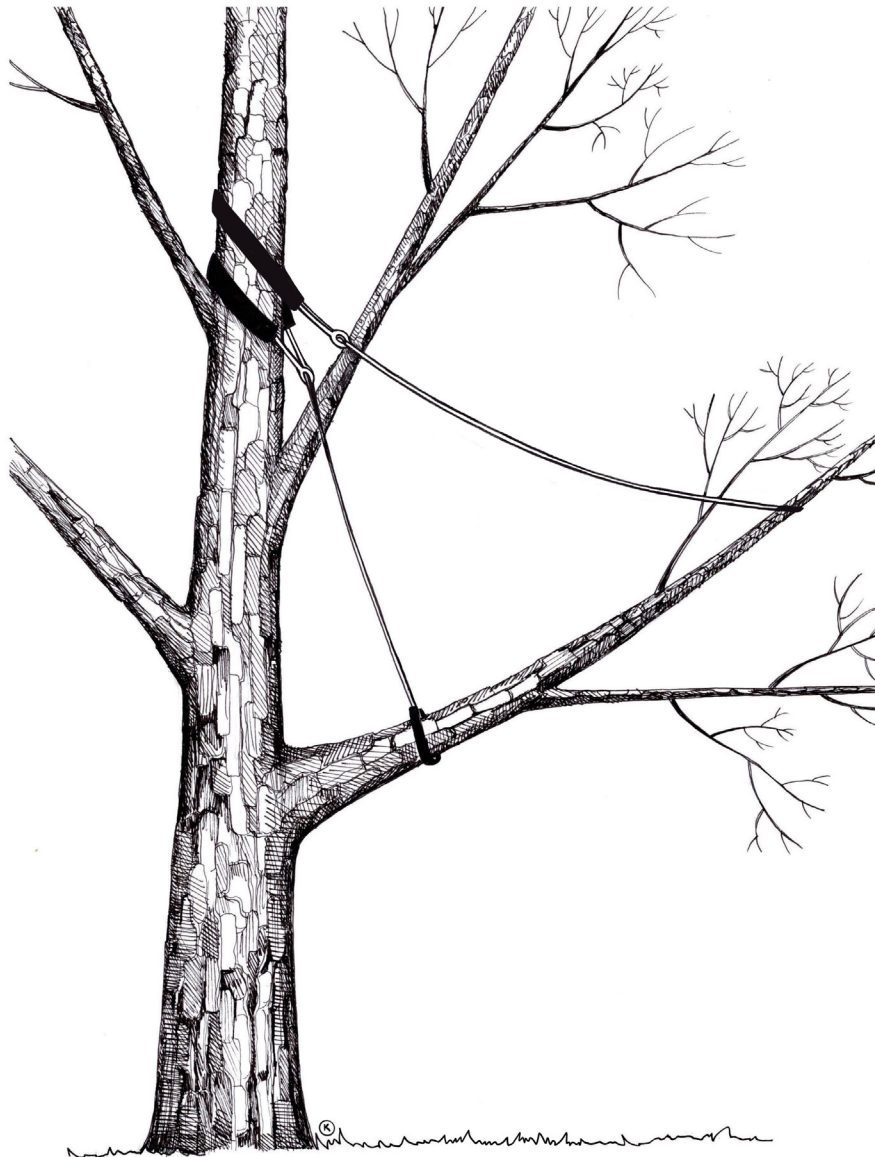
Figure 6: Securing a horizontal branch to prevent damage in the event of failure
